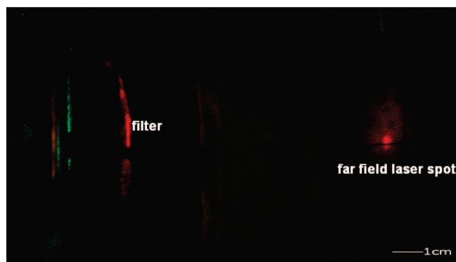
Figure 8. Far field image of the laser beam detected at 12 cm away from the microcavity.
